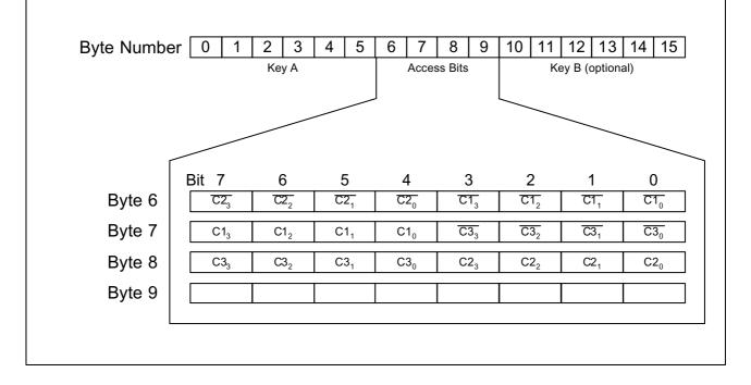
Note: With each memory access the internal logic verifies the format of the access conditions. If it detects a format violation the whole sector is irreversible blocked.
